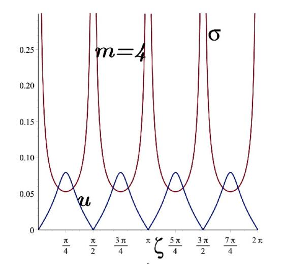
As one observes  $U_4 > U_3$  which implies that adding more cusps to the throat increases the energy needed. This is partly due to the fact that the total length of the hypocycloid is increasing as m increases such that  $\ell_m = \frac{8(m-1)}{m}$  with B = 1. This pattern goes on with m larger and in general
