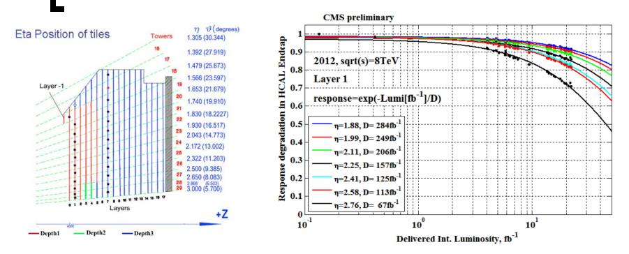
Degradation of signal in CMS HCAL Endcap in 2012 for the first sampling layer. A signal reduction of ~ 30% is observed at the highest pseudorapidity region ( $\eta$ =3).
