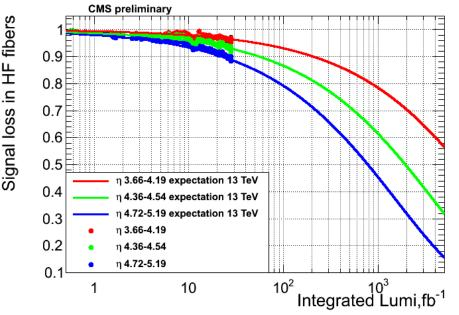
Expected loss of signal for up to 3000 fb<sup>-1</sup> In the highest  $\eta$  region, signal reduction by factor x3-x4 is expected and can be compensated by re-calibration.
