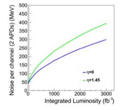
As a consequence there will be an increase in noise in EB. This increase would worsening the needed capability of rejecting spikes at trigger level.
