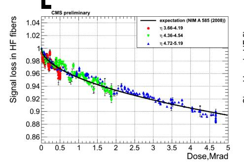
Signal loss in HF due to the radiation induced reduction of quartz fiber transparency.
